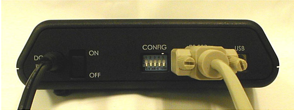
Figure 1-7 RS-232 Cable Connection
