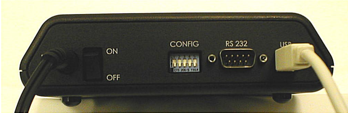
Figure 1-6 USB Cable Connection
