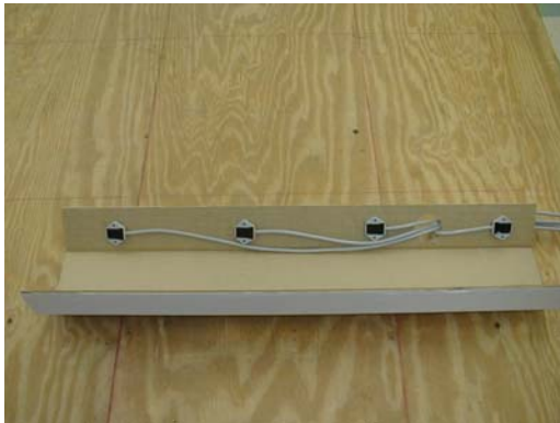
Figure 2 Placing Sensors in the QWIK-MAP pole
