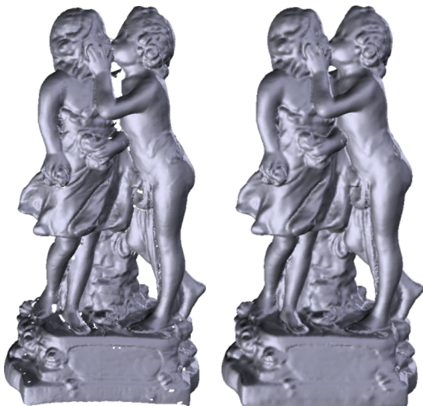
Figure 1: A FastSCAN™ scan (left) and the FastRBF™ surface (right). Small holes in the data, and the large gap between the embracing figures, have been filled automatically and smoothly. The topology of the statue (such as the gap between the hand and the throat) remain unchanged.
