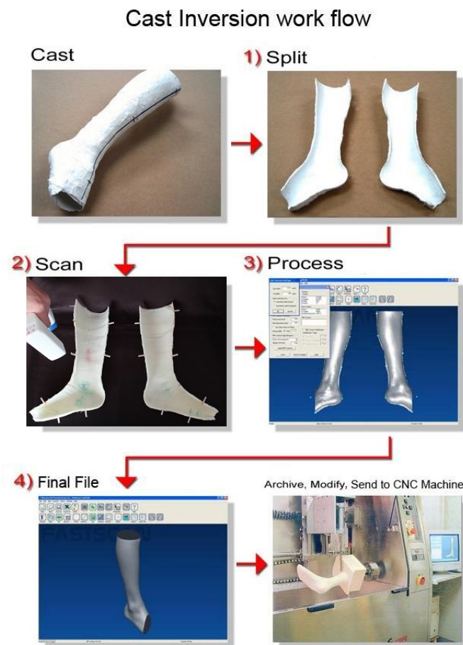
The process of scanning a plaster cast
