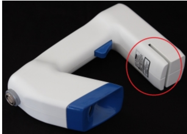
The Wand with product label and laser aperture circled.
