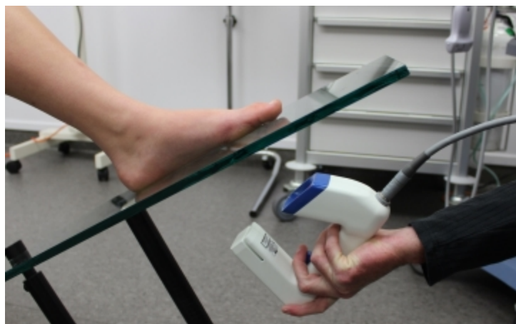
Scanning the base of the foot through glass.
